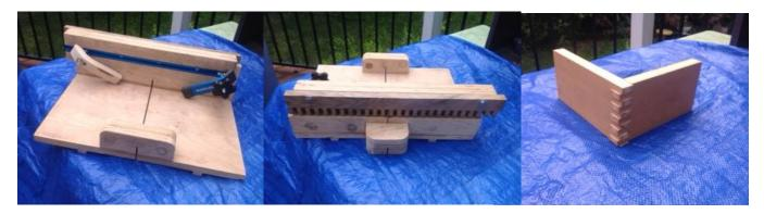
I finished making this box joint jig yesterday and tried it out this morning. It allows you to make any size box joint you want using a single, general purpose, table saw blade. The example shown in the picture is a 3/8" box joint corner. The jig is very easy to make and apparently it works fine. Keep on doing those wonderful NL's.
