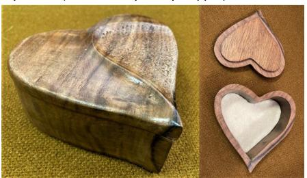
Roy's heart shaped bandsaw box he showed at the April meeting is Walnut. The lid was shaped with chisels and textured with a handmade tool. The texture tool is a door hinge pin filed on the end with a V shaped file. He hammered it in for texture. The box is finished with poly. It was a gift for his wife Pearl, on her Birthday this last week.
