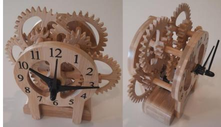
Here's my April Project Challenge entry. The clock uses an Arduino Nano processor and a custom motor driver to power a small stepper motor. The motor drives a sweep second hand with the gears providing a 60:1 ratio for the minute hand and a 12:1 ratio for the hour hand. Everything was cut on a CNC router using a 1/8" downcut spiral bit at 60" per second. Bamboo has a nice grain pattern without showing any tendency to
