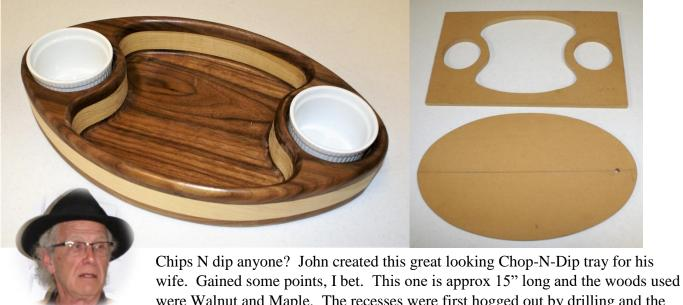
were Walnut and Maple. The recesses were first hogged out by drilling and the outer shape was cut on the bandsaw. Then with the aid of the templates shown, he was able to use profile router bits to refine the shapes. Note, due to the length of the shaping bits, he found it necessary to route using his router table. A round-over bit was used to ease all the edges.
