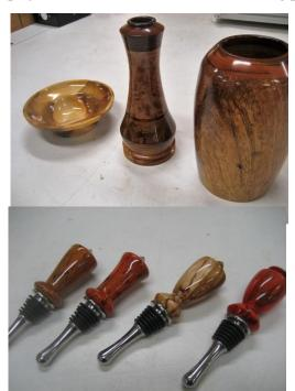
Far left: CA was used to harden soft end-grain for final turning, sanding and finishing.
