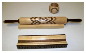
Rob took on the Celtic Knot challenge making the rolling pin and the napkin ring. The rolling pin holder was created using a parallelogram jig on the table saw. This can be a challenge as it requires many passes over the saw blade at an angle. A little sanding and you have a nice wide cove. Gee Rob, how about a demo.
