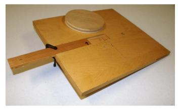
Homer showed his circle jig he uses on the band saw. He is able to set desired radiuses by sliding & clamping the slider with the circle center pin. This jig must be clamped to the band saw table with the blade gullet even with the center pin.
