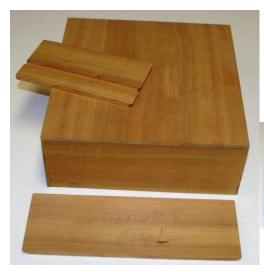
Ron brought in an example of a recessed lid joint box. Included were examples pieces with the groove layout required to have a successful lid to box to bottom fit. A project from Woodsmith "Ribbon Box handle" that uses this box top to bottom jointing method is attached to the email distributing this newsletter.
