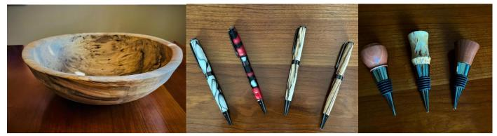
The above salad bowl of spalted Maple and measures 13 1/2 by 4 1/4. It and is finished with mineral oil and beeswax. For the ballpoint pens; two are acrylic; one is Spalted Maple, and one Zebra wood. For the three bottle stoppers: two are Madrone and one is Masur Birch from Finland. The pens and bottle stoppers were turned for a friend's church fundraiser.
