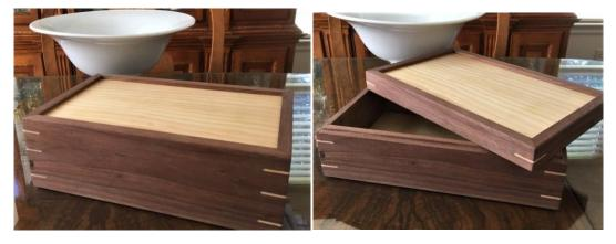
This box I showed at the July meeting is made using Walnut with a Pine top panel. The finish is shellac and the interior has black flocking. Centrifugal force is used to release the top. Spinning the box forces brass rods mounted in the base in opposing directions leaving the catches in the center of the top free, therefore allowing the top to be removed. The pictures are from early in the box development as the box has been presented to a birthday girl.
