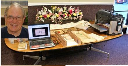
Member John Cope brought in a system that is used to create patterns he uses in recreating items with CNC machine. The system is made up of a computer and a scanner unit. The scanner looks much like one of our small planner machines and is used to create digitized images he wants to send to the CNC machine. He explained how he sets up the target item to be scanned by mounting it in a carriage. The
