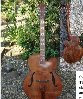
I finally finished this guitar, it took forever. The top (soundboard) is from a 2' slab of old growth Redwood that was resawn into two 1" boards then book matched. The book matched boards were band sawed to profile. The top was carved to a dome shape then the underside of the top was scooped out resulting in a top thickness that ranged from 1/4" down the center to 3/32" near the edge.
