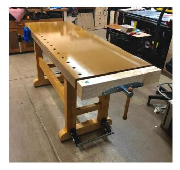
Here is the photo of the workbench I showed at the last Zoom meeting. The top is 3" thick MDF, finished with 4 coats of Minwax Tung Oil Finish, applied with a roller. The end vise is by Sjobergs, to which I added a 3" thick Birdseye maple chop. The side vise is an old Wilton Sheldon quick release vise that I restored. The bench weighs about 200 lbs and has retractable casters from Rockler, attached together with 3/4" steel tubing.
