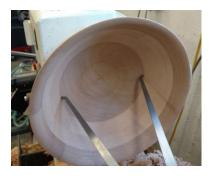
• Reverse bowl and mount in large face chuck.. Pare off tenon and finish bottom
