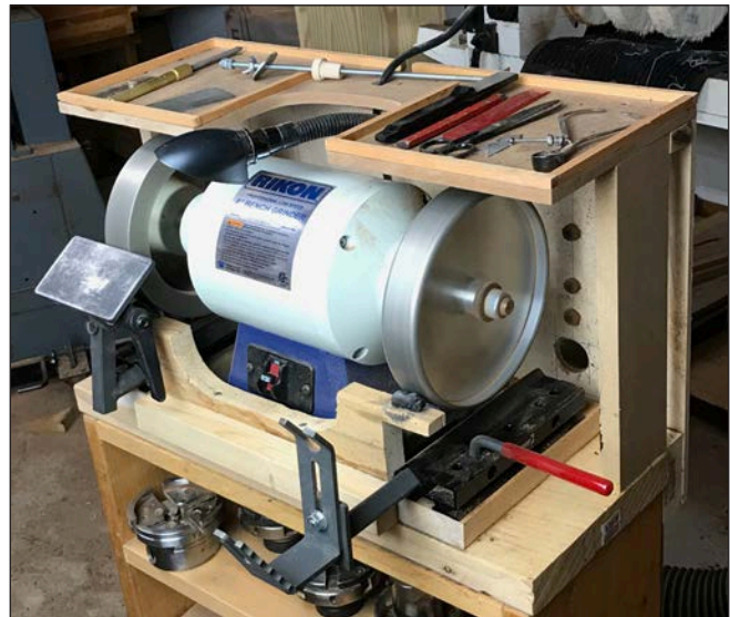
Shopmade grinder stand holds tools and keeps forehead and CBN wheels safely separated.
