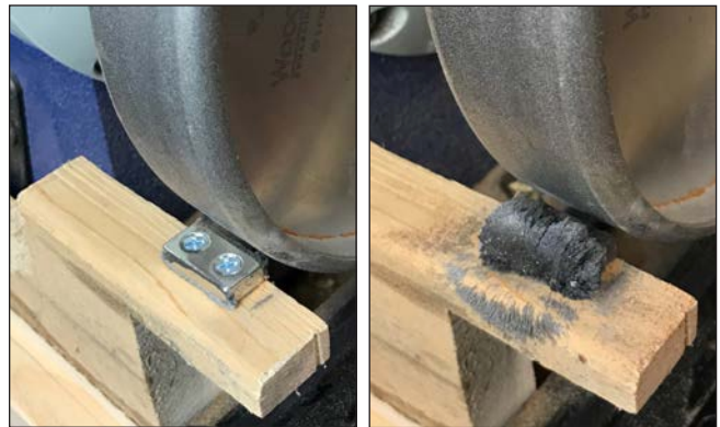
Bar magnet mounted below the CBN wheel (left) captures metal particles (right).
